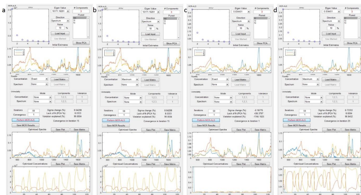
Figure 23. The effect of Concentration Equality Constraints. The example uses the “demo_image.txt” file exactly as in Figure 19 for a and b , and with Total Area Normalisation for c and d . 3 components are selected for MCR-ALS, using automatic initial estimate determination, spectral direction and 10% noise. Convergence limit is set to 1 for speed, and maximum number of iterations is kept at the default 50. Results are identical without normalisation (c.f. a and b ) since the constraints are numerically outside the range of the dataset (see the scale on the Y-axis of the Optimal Concentration Plot). For visualisation purposes, either the csel matrix values need to be adjusted, or the spectra scaled, by e.g. total area normalisation. This highlights the effect of the concentration equality constraint and the differences between “equal” (a hard constraint) and “maximum” (a milder constraint), c.f. c and d .
