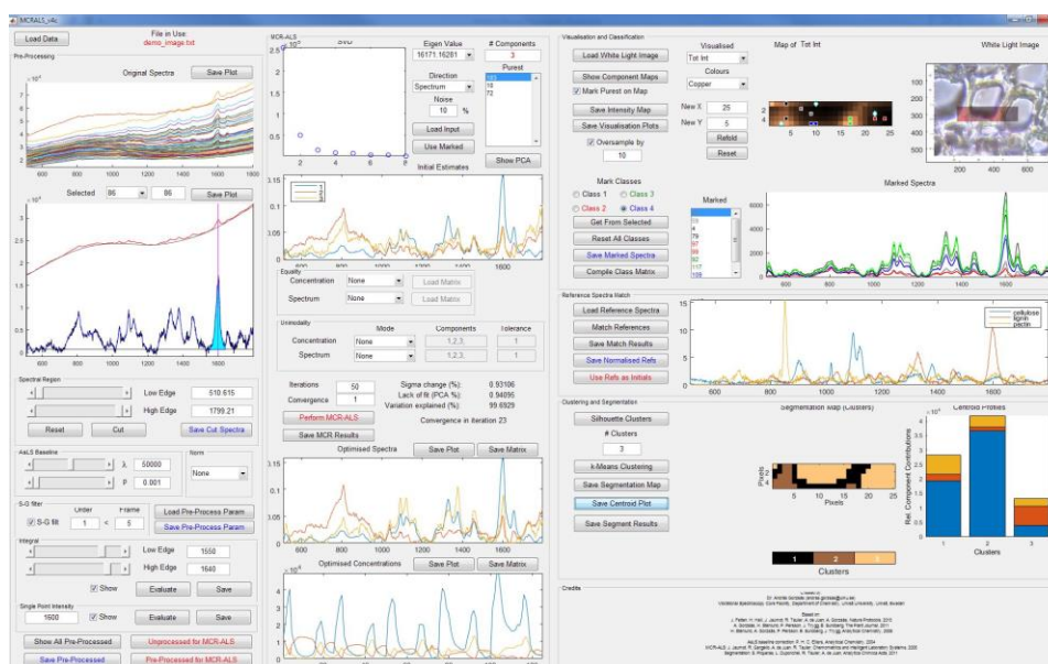
Figure 36. The fully populated GUI. The example uses the “demo_image.txt” file after MCR-ALS imaging (as described in Figures 16 and 26 ), with the “demo_references.xlsx” auxiliary dataset loaded. Classes are marked as in Figure 31 , and segmentation performed after silhouette clustering with 3 clusters ( Figure 35 ).
