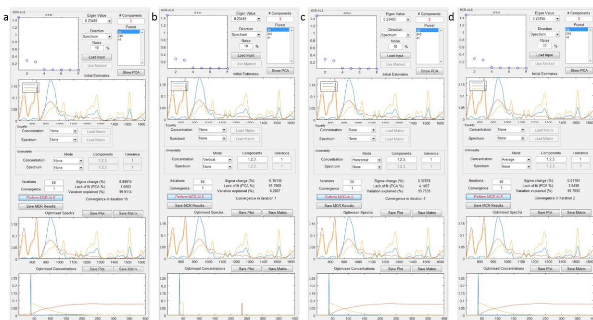
Figure 25. The effect of Concentration Unimodality Constraints. The example uses the “demo_series.mat” file, with the following pre-processing parameters: spectral region cut to 700 – 1630 \text{cm}^{-1} ; \lambda=10,000 and p=0.001 ; No Normalisation and Savitzky-Golay smoothing with 1 st order polynomial and Frame=5. 3 components are selected for MCR-ALS, using automatic initial estimate determination, spectral direction and 10% noise. Convergence limit is set to 1 for speed, and maximum number of iterations is kept at the default 50. Results are shown with no unimodality constraints (a), and concentration unimodality constraints (vertical, b, horizontal, c, and average, d) for all 3 Components. Note that apart from the vertical constraint (b), all results are very similar, achieved in much fewer iterations with the constraints.
